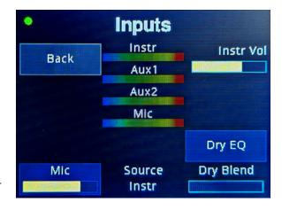
• Turn **Source** to change from Instrument input to Aux input. Aux input can operate as a normal mono input, or it can be a stereo dual-source input.
